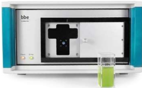
Figure 17: bbe fluorometer, chlorophyll-a determination
